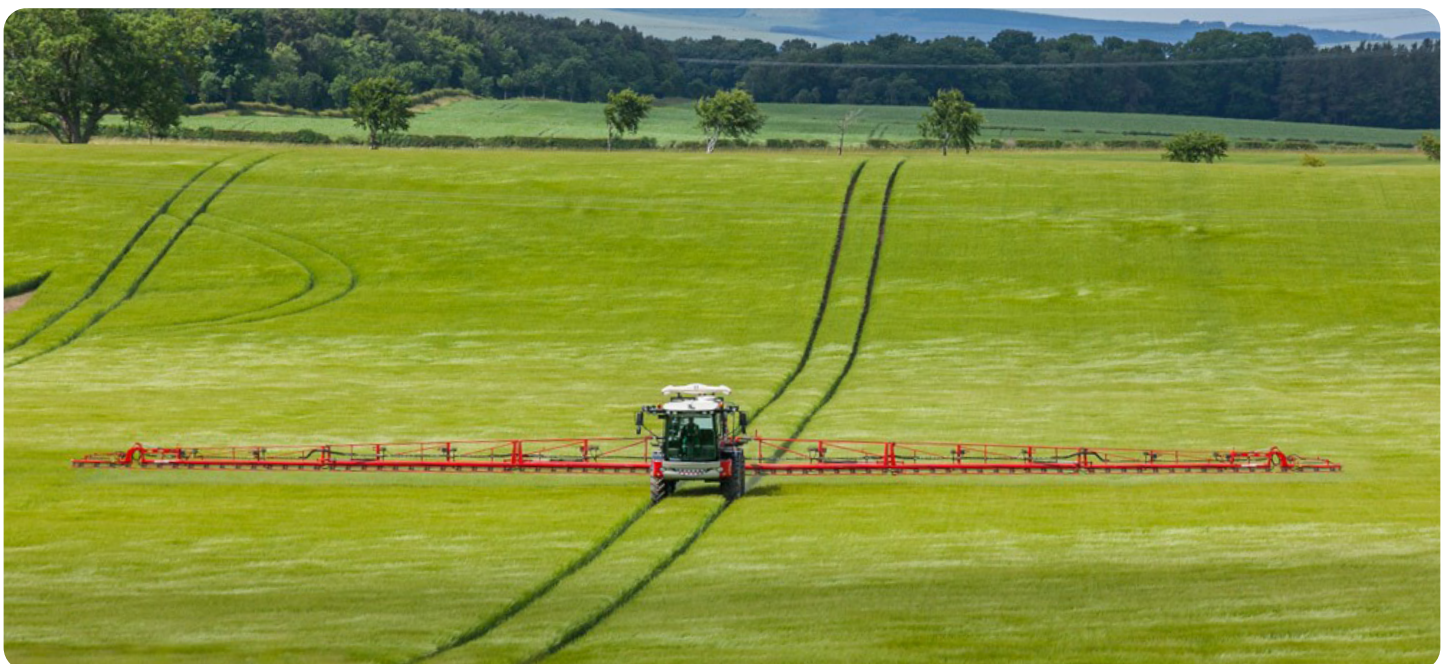
A crop sprayer travels up and down fields using tram lines. The tramlines are placed at set distances apart in the field to ensure that there is no overlap of the spraying zone.
